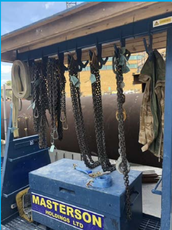
Good-quality storage of lifting accessories to be established and maintained
