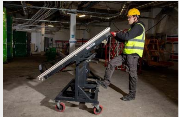
Rotating board trolley to provide safe storage and working bench
